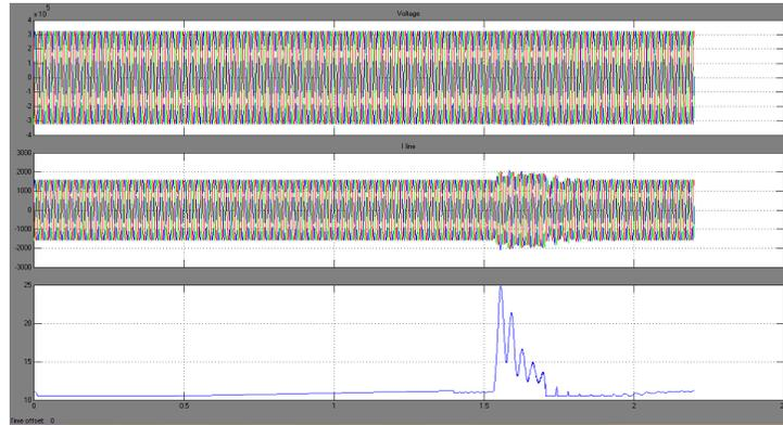
**Figure 8: (a) Voltage at the other end of the transmission line (b) Line Current I line(c) X reference for the control circuit**
