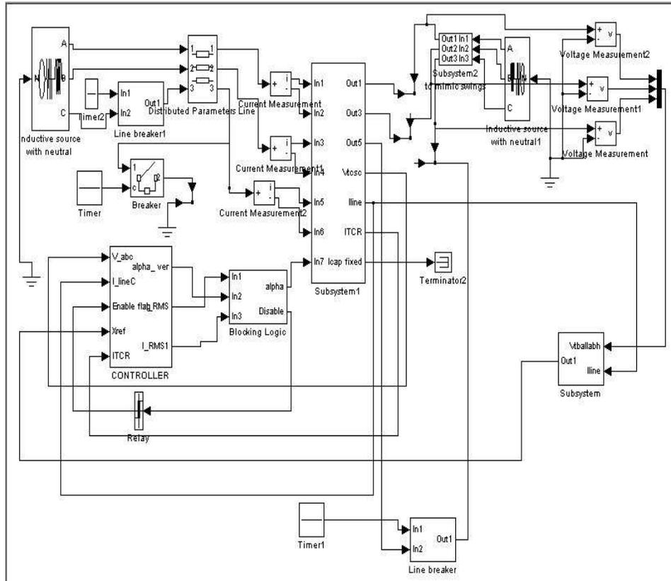
**Figure 4: 3-phase transmission line with TCSC**
