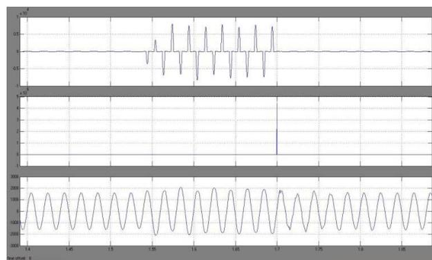
**Figure13: (a)1-phase Current through TCR (b) 1-phase Current through the Capacitor
