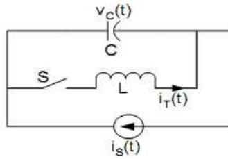
Figure 2: A Simplified TCSC Equivalent Circuit
